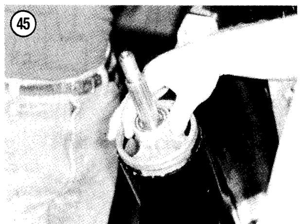
6. Install bearing carrier retainer wrench (part No. C-91-54873) and rotate counterclockwise to loosen the cover nut. Remove tool and turn cover nut out by hand. Remove nut and tab washer.
